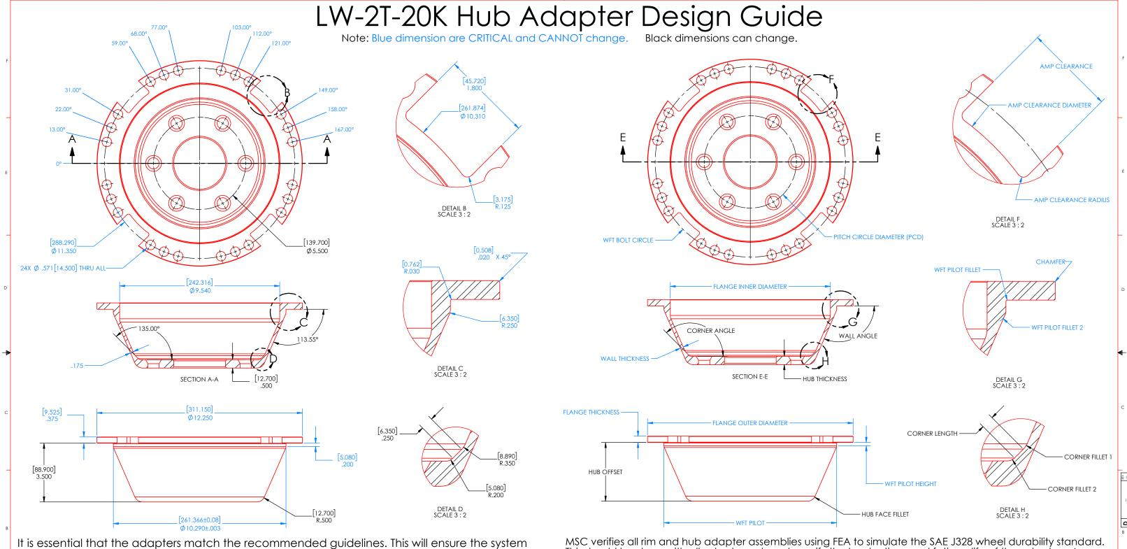
can withstand the rated loads and provide the most accurate results. The critical features are shown in blue. Customers may change all other geometry. Examples of permitted changes are shown on the second sheet.
